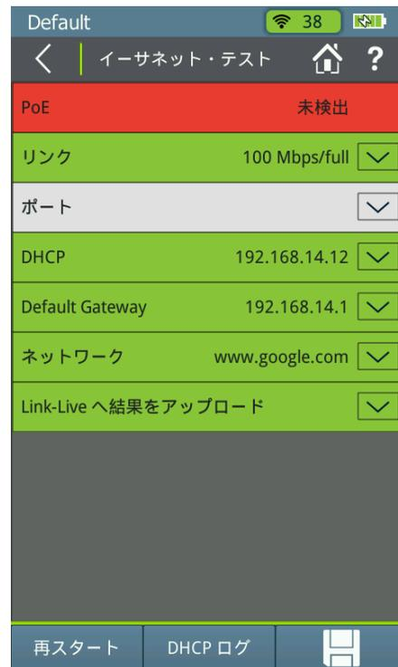
The screenshot shows the 'イーサネット・テスト' (Ethernet Test) screen in the AirCheck G2 application. The status bar at the top indicates 'Default' and 'Wi-Fi 38'. The main content area displays the following network configuration details:
