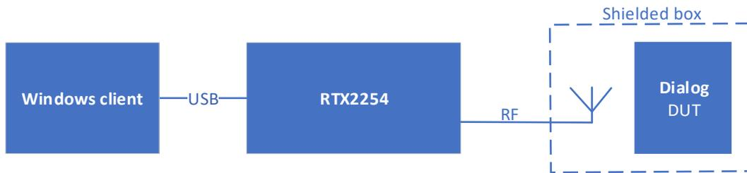
Figure 2: Using RTX2254 for test in Advertising mode
